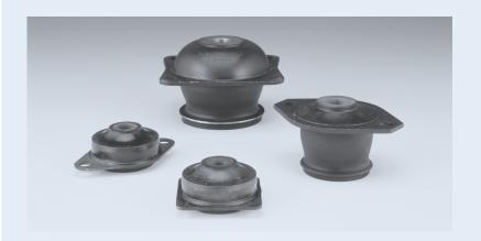
Industrial Conical Mount Series Isolators are designed to withstand the rigors of heavy-duty vehicular applications, off-road equipment, large trucks and construction equipment. They provide shock, vibration and noise isolation and are designed for high impact applications.
